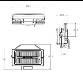
The second new addition to the TRALERT® Atlas driving light line: the Atlas 220+ block light (Art. WD-5860A). A modern version with duo-color daytime running lights of the classic and popular block lamp spotlight, to which this variant also adds an R65 certified LED warning light. With a light output of 6,000 lumens and retaining its classic design, this driving light is particularly suitable for giving your truck a contemporary look while greatly improving visibility and signalling.
