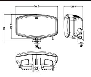
All functionalities in a popular format LED driving light: the TRALERT® Atlas 320+ (Art. WD-6060A). This LED driving light is equipped with powerful LEDs with a total light output of 6000 lumens. In addition, the Atlas 320+ is equipped with duocolor daytime running lights and an R65-certified LED warning light, making separate warning lights on your roof bracket unnecessary.
